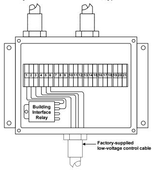
Figure 11 Main input junction box connections, typical
